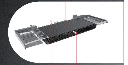
VARIABLE DAMPER to accurately control top temperature High Efficiency MESH BURNER
